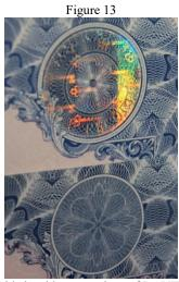
Side by side comparison of DOVID cycloid with key image compared to intaglio cycloid with same illumination
