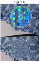
Side by side comparison of DOVID cycloid with lock image compared to intaglio cycloid with same illumination
