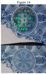
Side by side comparison of DOVID cycloid with word SAFE Image compared to intaglio cycloid with same illumination
