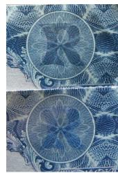
Side by side of two different intaglio documents under same illumination. Top image reflects good embossment relief and bottom shows effect of poor embossment relief.
