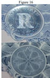
Side by side comparison of DOVID cycloid showing latent image R compared to intaglio with same illumination
