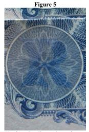
Hard to visually see latent image due to insufficient intaglio embossment
